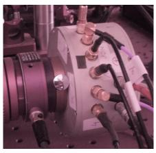
2) Automatic protection high voltage shutoff NIM module. Programmable high voltage settings and shutoff threshold (in max number of counts per second). Shutoff time – less than 75 ms after overflow:
